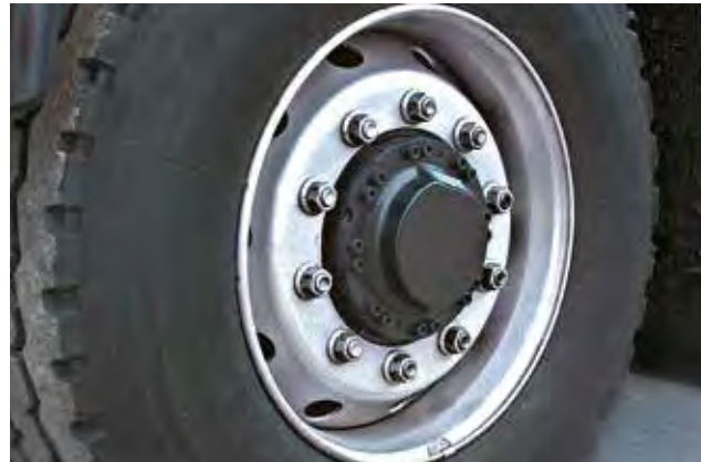
Front axle with hydrostatic wheel hub motors
